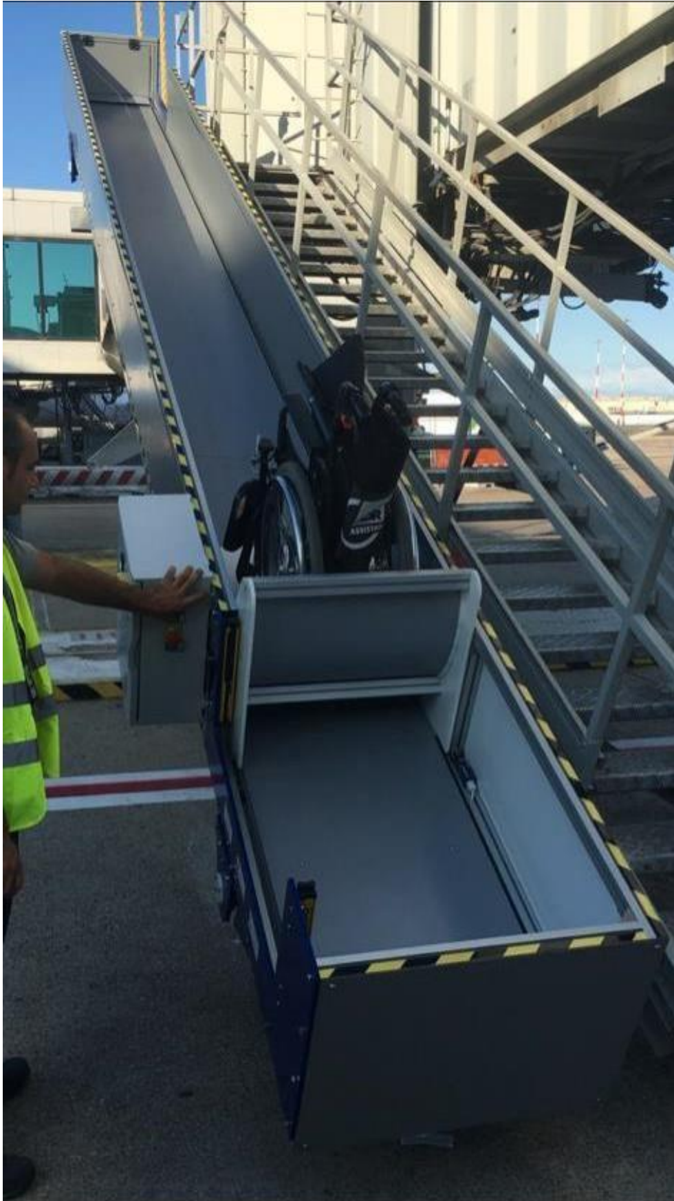
Image 7. The handler operates the button to raise the device from runway level to pier level
