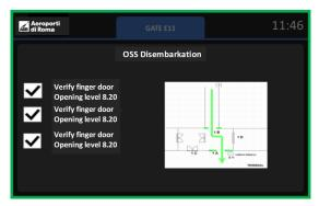
Having selected the OSS Disembarkation operation, the *glass door of the finger (B)* and the *glass door of the gate (A)* open.
